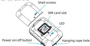
Key Description: Press and hold the power button for 3 seconds to turn on/off;Non-shutdown version (factory default setting)
